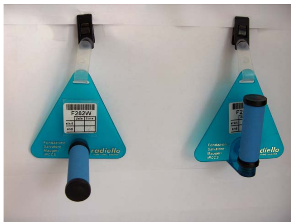
Figure 6.3: Supporting plate for the Radiello sampler
